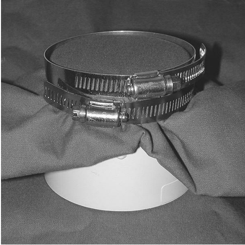
Figure 2. Fabric clamped onto flange with two hose clamps. Notice that the second one will protrude a bit above the level of the fabric with thicker fabrics, but it should still be tight if you push everything down enough.
